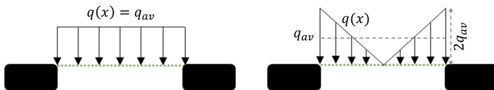
Figure 2.20 – Uniform and inverse triangular load distributions on the GR in the Dutch CUR 226 guideline
