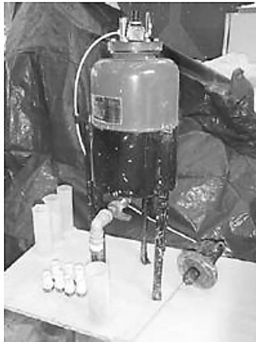
Figure 33. Penetrability meter (Eriksson and Stille, 2003).
