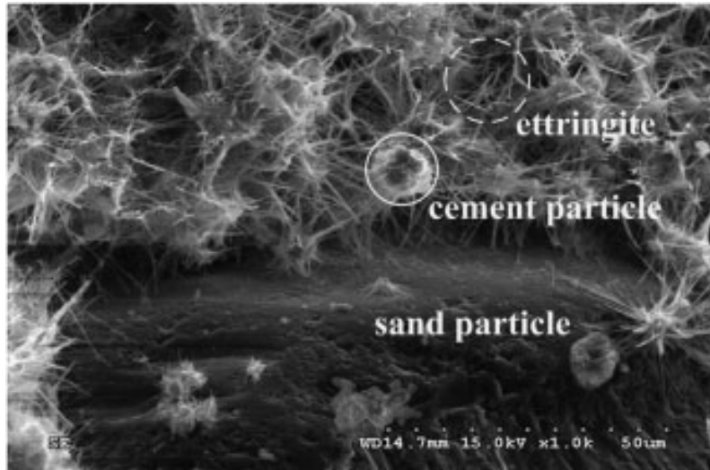
Figure 6. Formation of ettringite in the cement-based grout (Kim et al.,2009).
