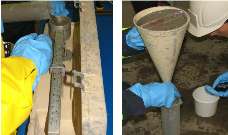
Figure.21, Mud Balance test device for measurement of the density (left) and Marsh cone (right) for measurement of Marsh value (Ranta-Kopri, et al., 2008).
