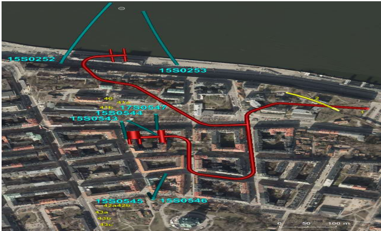
Figure 4.4. Londonviadukten access tunnel marked in red, and the core boreholes location is indicated in blue (FUT,2019).
