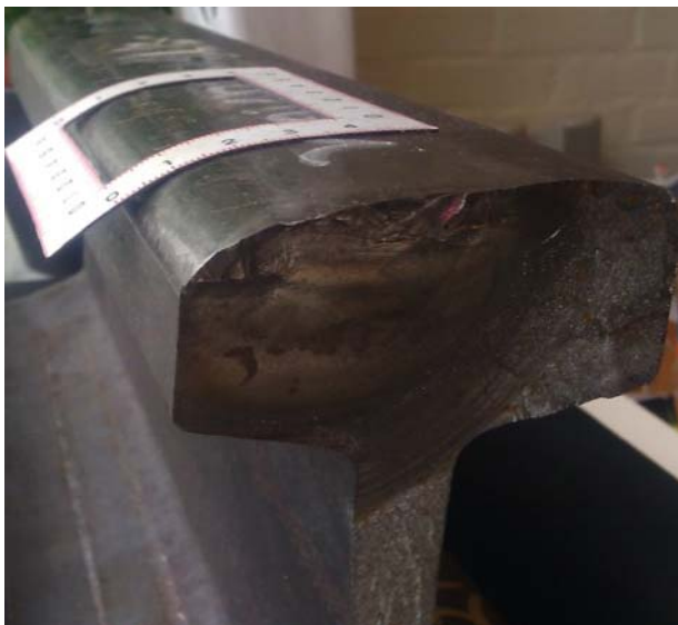
Rail break setting out from a headcheck crack
